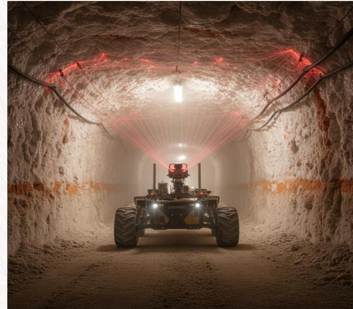
Autonomous robot-mounted Hovermap – navigating a hazardous potash mine drift, hands-free
